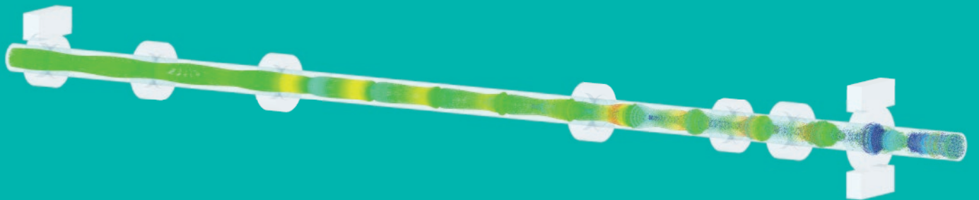
Particle trajectory in a klystron: A PIC Solver simulation of a 1.24 m klystron. The bunching which produces the RF signal is clearly visible.
